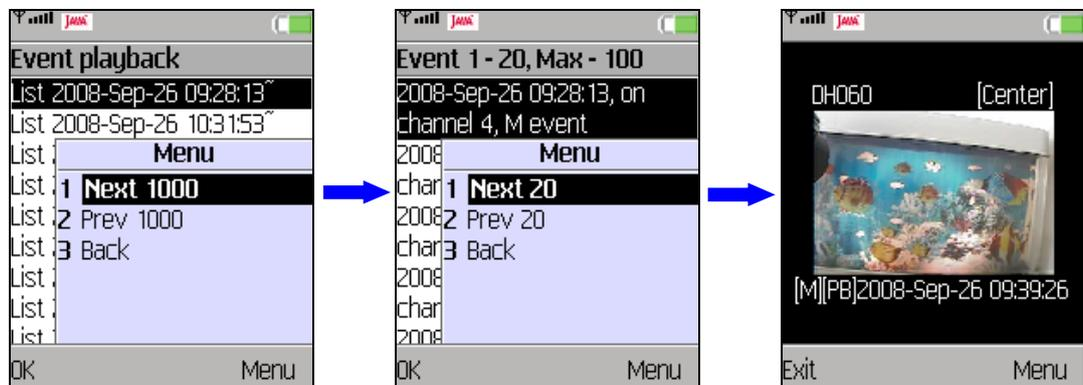
Each page of the list contains 20 events. Press <Menu> and select <Next 20> or <Prev 20> to show a different page. Press “UP/DOWN” key to scroll through the events and press <OK> to start the playback. As shown above, “[M][PB]” will be displayed in front of date/time at the bottom of the screen to indicate that it is currently in “Event Playback” mode. The first letter indicates event type, for example M=motion.
