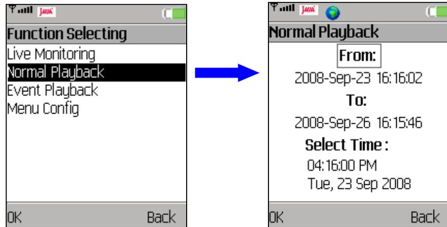
Press “DOWN” key to move selection box to time and date, then press “ENTER” key to set playback starting time and date, as shown below. After date and time are set, press <OK>. Then select a channel to start the playback. The text “[PB]” will be shown in front of date/time at the bottom of the screen to indicate that it is currently in “Normal Playback” mode.
