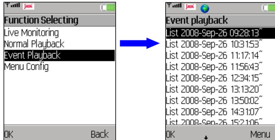
On the screen is an index of lists, which each contains 100 events. If the index contains more than 1000 lists, press <Menu> and select <Next 1000> or <Prev 1000> to surf faster. Press “UP/DOWN” key to scroll through the screen and select a list.
