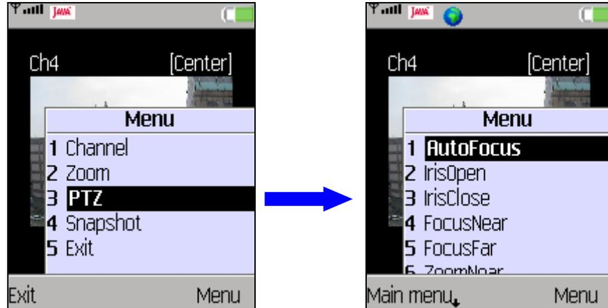
Press <Main menu> to exit dome camera PTZ control mode.
